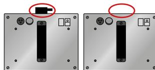
For removing the metal cover, remove the perimeter screws that secure the cover to the box, as shown in figure 02. During the operation, keep the cover pushed towards the box using the handle.
