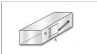
5. Draw the dimensions of the hole (225 x 145 mm) according to the model of the product using the template provided for the BXMC series.
