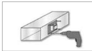
6. Use a jigsaw or cutters to remove the marked section of the duct and remove sharp edges. Place the BioxAir device on the side of the air duct and screw.
