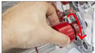
2. Screw the quartz condenser rotating the red plastic bushing at the base.
