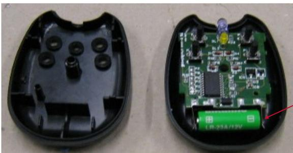
To replace the remote control battery:
